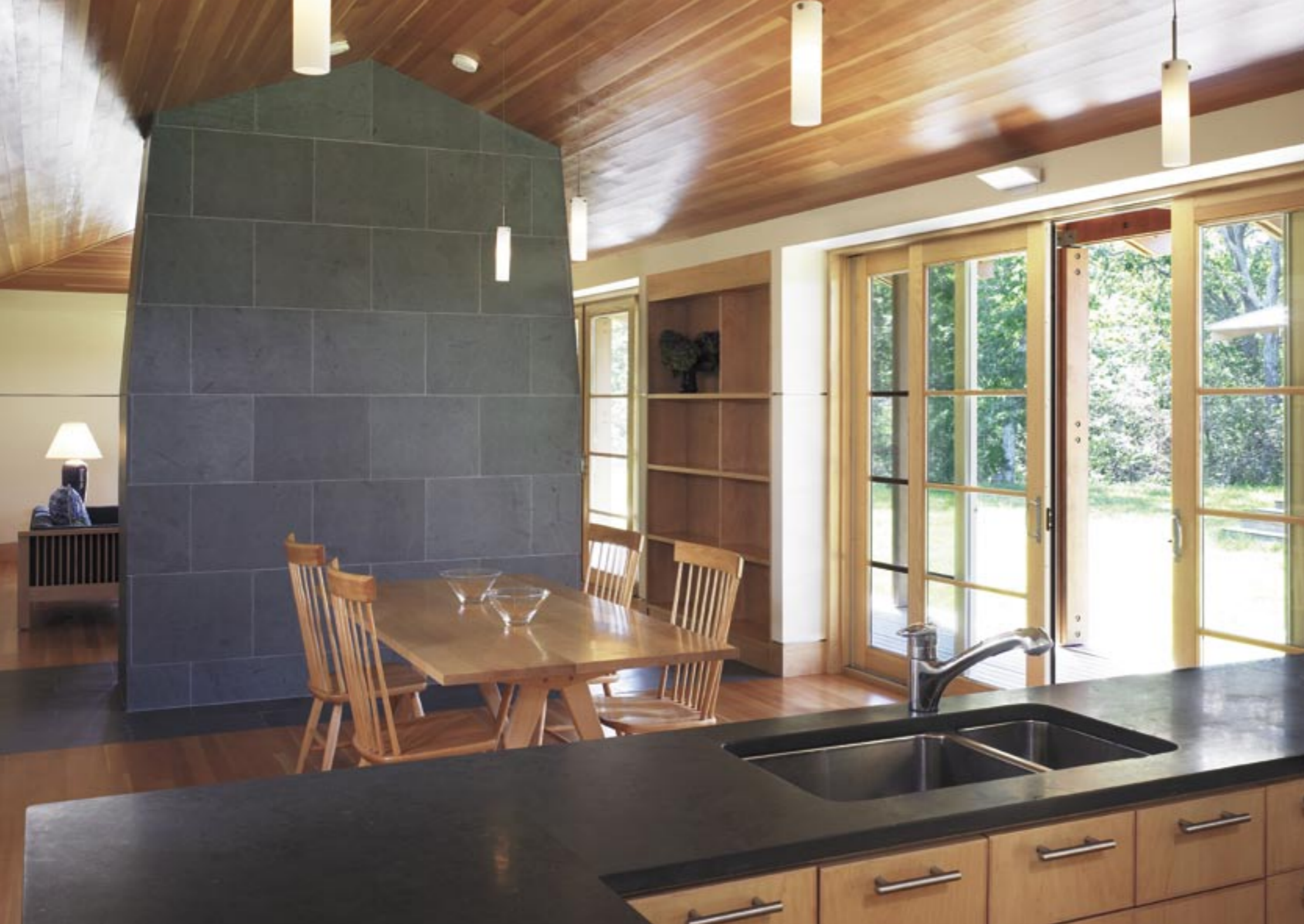
Above and right: The living room fireplace uses a Rumford-style firebox designed to maximize energy efficiency. The chimney and the surrounding stone floor are designed as a thermal flywheel – absorbing heat during the day and re-radiating it at night. All living and sleeping areas open out through large doors to wide porches and the grass-covered central space.
